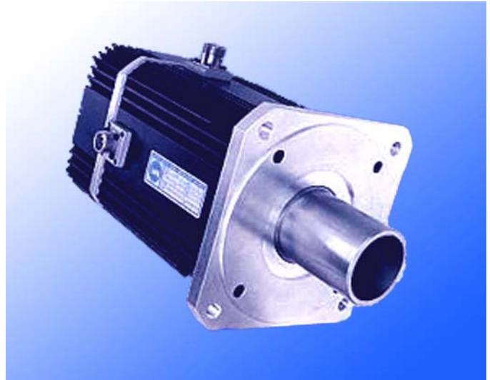
Like a conventional AC motor, the stator coil is supplied with sinusoidal, three-phase AC-current. At PWM control of the circulation frequently and the terminal voltage, the speed of the SynchroDyn servo motor can smoothly operate between zero speed and max. no-load speed, in addition high rated and maximum torques are available over the whole speed range.
